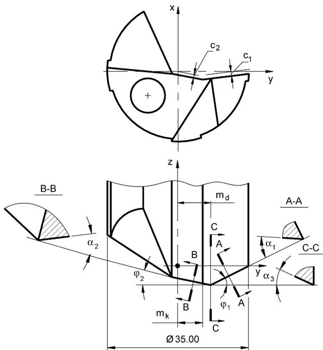
Fig. 1. Design parameters of a gundrill.
