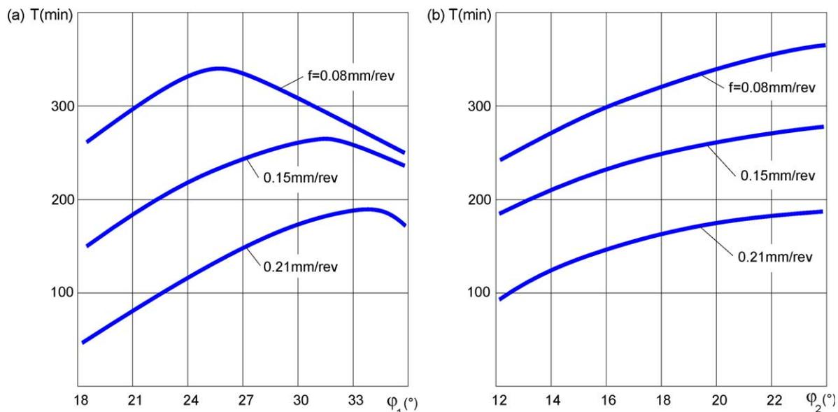
Fig. 5. Tool life  $T$  vs. (a) the approach angles of the outer cutting edge,  $\varphi_1$  and (b) the approach angle of the inner cutting edge,  $\varphi_2$  for different feeds.
