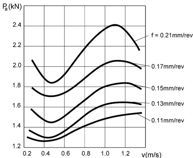
Fig. 2. Influence of the uncut chip thickness (the cutting feed,  $f$ ) on the axial force,  $P_a$  under different cutting speeds,  $v$ .
