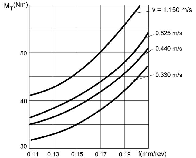
Fig. 3. Influence of the uncut chip thickness (the cutting feed,  $f$ ) on the drilling torque,  $M_T$  under different cutting speeds,  $v$ .
