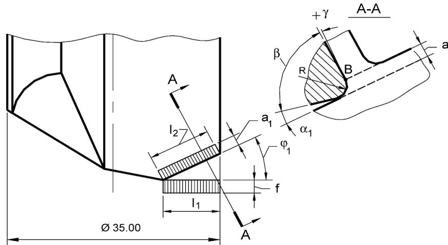
Fig. 6. Model showing influence of the approach angle of the other cutting edge  $\phi_1$  on the uncut chip thickness (the chip load)  $a_1$ .
